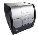
**BioTek Cytation 5 multimode plate reader and imager:** This reader provides Tempus with the flexibility to provide information on NGS quantification, well-based quantitative data, and automated phenotypic cellular information up to 60x magnification.
